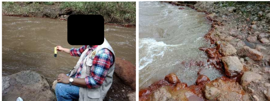
FIGURE 2. The pH measurement of Banyupait river water (left image). The river's ground rocks have oxidation due to acidic water reactions (right image).
